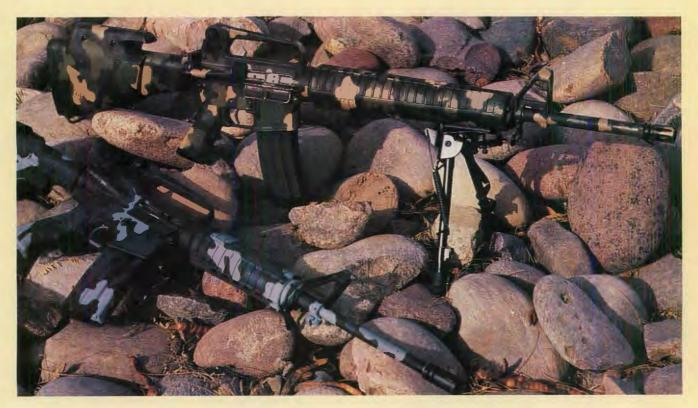
als and alloys, providing the appearance of satin electroless nickel by combining sub-micron particles of PTFE with autocatalytically applied nickel-phosphorus. The result is a very accurate, drylubricated, lowfriction surface Two Colt AR-15s after Polymax treatment; the rifle in woodland camouflage, the carbine in an urban pattern. Polymax provides excellent resistance to water, many corrosive chemicals, abrasions and impact.
